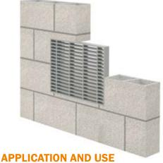
Tecsel® Grilles are mechanically attached to the supporting constructive element with the appropriate screws, plugs or fittings (these must have at least the same level of fire resistance as the structure onto which they are fixed).
