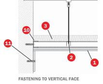
it with the 40 mm and 40 kg/m<sup>3</sup> rock wool above the structure. Then, place the second board layer using 3.5x45 mm self-tapping screws alternating it with the first layer.
