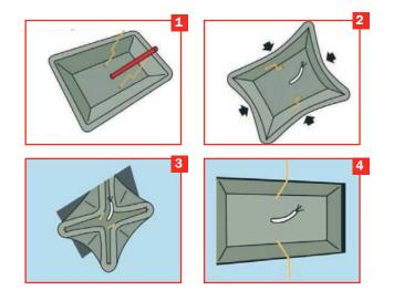
\* In a wall with two layers of plasterboard on each face, the ends of the fixing wires can be pushed between the plasterboard layers.
